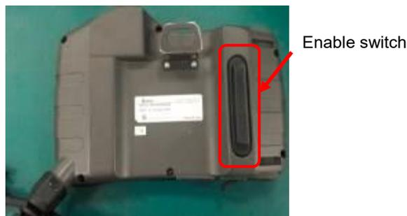
Figure 8.31 Location of the enable switch on the teach pendant
