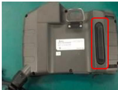
Figure 7.46 TP Enable switch icon
