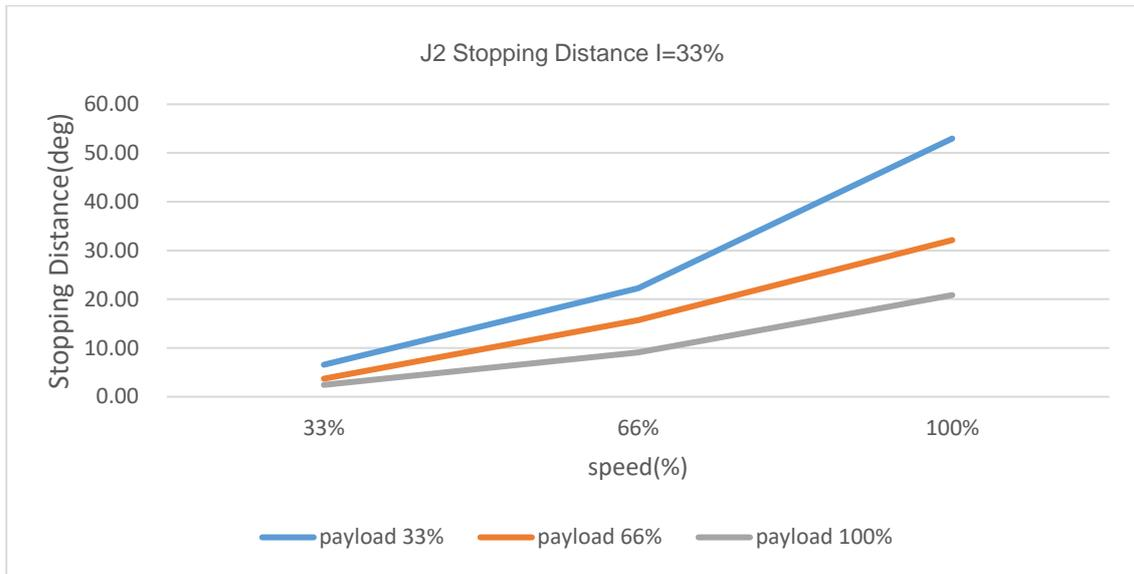
Figure 3.36 J2 Stopping Distance (DRV70L Extension 33%)
