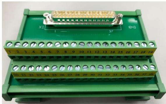
Figure 12.8 External encoder conversion module
