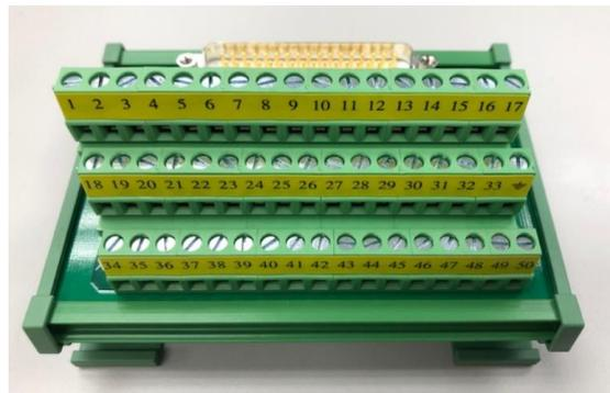
Figure 12.4 Standard DI/O conversion module
