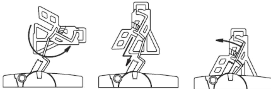
Figure 8.39 Circuit breaker lockout device
