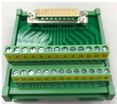
Figure 12.4 System DI/O conversion module
