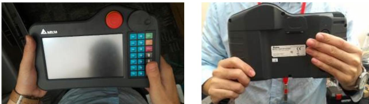
Figure 7.47 Correct way to hold the TP
